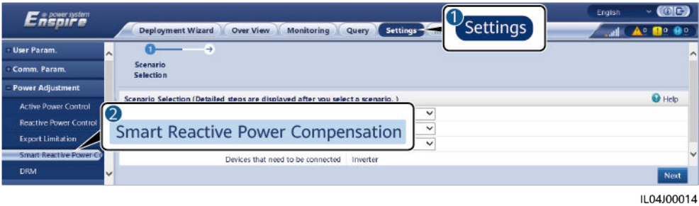
Figure 6-79 Setting parameters for smart reactive power compensation (Scenario Selection)
