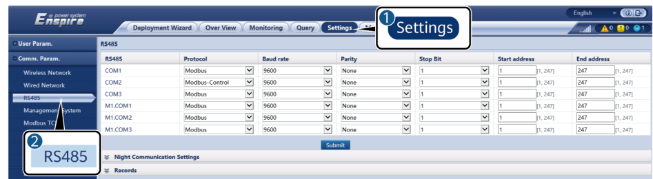
Figure 6-87 Setting RS485 parameters
