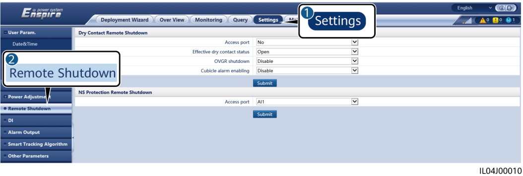
Figure 6-86 NS protection remote shutdown
