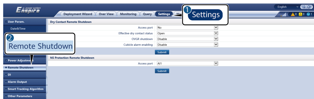
Figure 6-84 Dry contact remote shutdown
