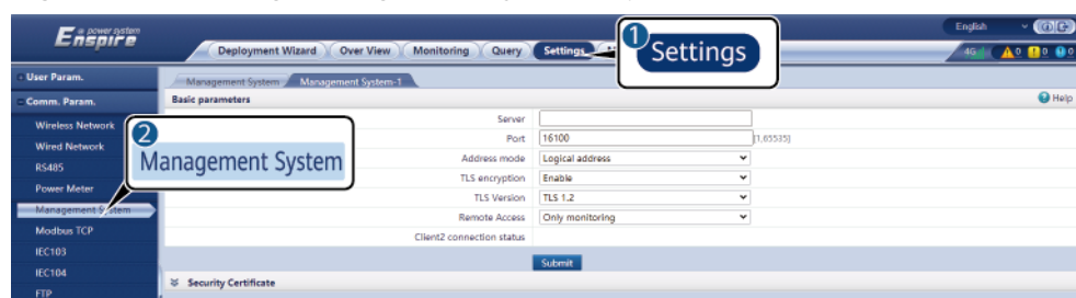
Figure 6-31 Setting management system-1 parameters
