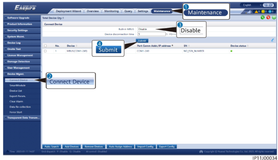
Figure 6-45 Setting parameters for a built-in MBUS module
