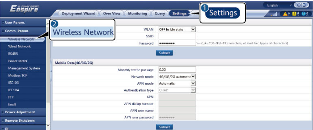
Figure 6-28 Setting mobile data parameters
